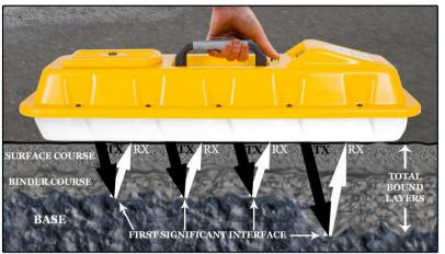
The e-Spott is an advanced system designed specifically to measure the Total Bound Layer Depth of asphalt surfaces such as those typically used for footways and minor carriageways.
