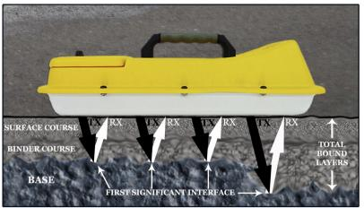
The e-Spott<sup>HF</sup>is an advanced system designed specifically to measure the Total Bound Layer Depth of asphalt surfaces such as those typically used for footways and minor carriageways.
